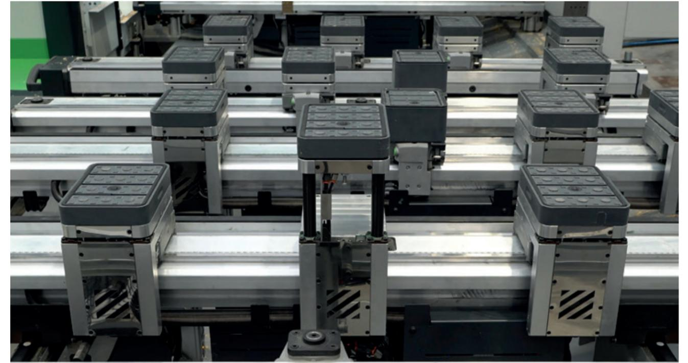
"A Hyperpod is a standard pod that allows you to lift and lower workpieces so secondary operations can be carried out."
